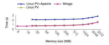
Figure 5: Domain boot time comparison.
