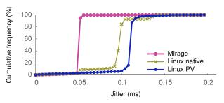
(b) Jitter for  $10^6$  parallel threads sleeping and waking after a fixed period.
