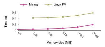
Figure 6: Boot time using an asynchronous Xen toolstack.
