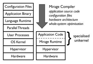
Figure 1: Contrasting software layers in existing VM appliances *vs*. unikernel's standalone kernel compilation approach.
